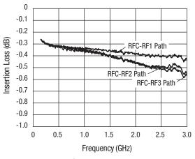
**Insertion Loss vs. Frequency**
