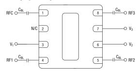
$C_{BL} = 47 \ \text{pF}$  for operation  $> 500 \ \text{MHz}$ . Exposed paddle must be grounded.
