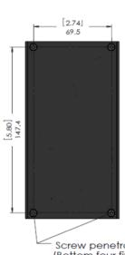
Screw penetration 3.0mm Max. (Bottom four fixed hole)
