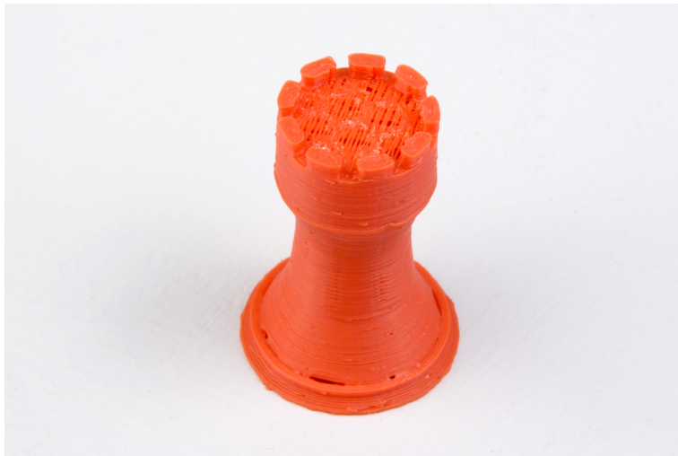
Figure 2.15: An example of insufficient top layers.
